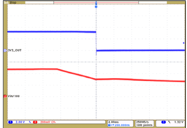
Figure 28 Shut Down V_{IN} Vs V_{OUT} ( V_{IN} = 48V I_{OUT} = 18A C_{OUT} = 12X10\mu F X7R Ceramic)
