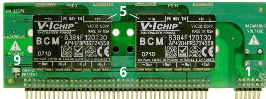
Figure 2 High Voltage BCM Series Array (back)
