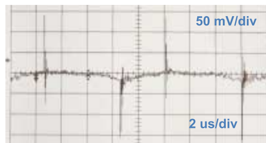
4(a) Conventional 100 kHz PWM Forward
